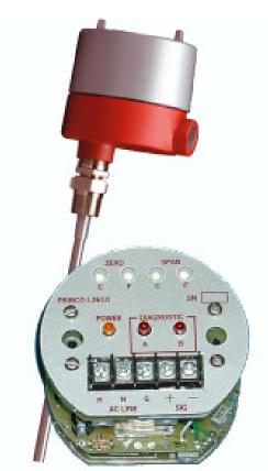
PRINCO's L2610 NULL-KOTE™ four-wire RF level transmitter can be used to measure the level of virtually any process material, from low-dielectric (insulating) products, such as refined oils, to conductive slurries— even viscous materials that cling to the probe.
